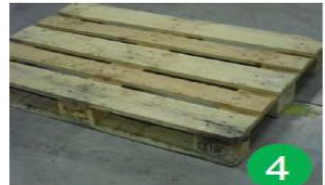
9 Poor general condition of the pallet: - major contamination (e.g. lubricants, grease, cement) - use of impermissible elements – boards, bearers, nails - improper positioning of the elements, e.g. bearer moved versus boards
