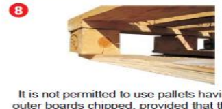
8 It is not permitted to use pallets having their outer boards chipped, provided that the depth of the chipping exceed 2 cm and more than 1 nail is visible.
